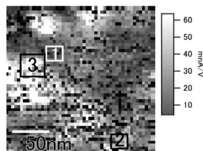
Fig. 3.  $dI/dV$  image for sample voltage of 0.8 V.
