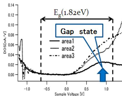
Fig. 2.  $dI/dV$ -V curves for each squared area drawn in Fig. 1.  $E_g$  denotes bandgap of pentacene.
